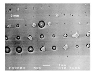
**Fig.5.** SEM overview image of damage topographies of diamond turned  $CaF_2(111)$  surface irradiated with the fluences in range from 18.3 to 55.3 J/cm<sup>2</sup>. White spots represent surface damage, *dark halos* originate from recondensed plasma debris
