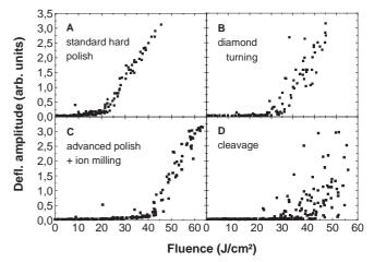
**Fig. 1a–d.** Fluence dependence of the photoacoustic signal amplitude for differently prepared (111) surfaces of  $CaF_2$  crystals. **a** conventional standard polish; **b** surface prepared by diamond turning; **c** chemo-mechanical polish; **d** cleaved surface
