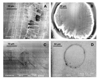
**Fig. 4a–d.** SEM images of damage topographies of fluoride surfaces polished by diamond turning and irradiated with the following fluences: **a** CaF<sub>2</sub> - 36 J/cm<sup>2</sup>; **b** LiF - 50.4 J/cm<sup>2</sup>; **c** BaF<sub>2</sub> - 12.6 J/cm<sup>2</sup>; **d** MgF<sub>2</sub> - 54 J/cm<sup>2</sup>. The laser spot diameter is 100  $\mu$ m in all cases. Notice the magnified scale in a and c
