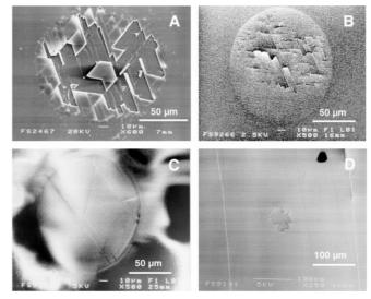
**Fig. 2a–d.** SEM images of damage topographies of  $CaF_2(111)$  surfaces irradiated with the following fluences: **a** 27.6 J/cm<sup>2</sup> at the conventional standard polish; **b** 30 J/cm<sup>2</sup> at the diamond turned surface; **c** 57.7 J/cm<sup>2</sup> at the chemo-mechanically polished surface; **d** 46 J/cm<sup>2</sup> at the terrace area of a cleaved surface
