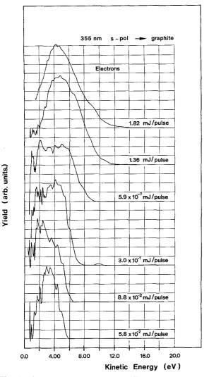
Fig. 3. Electron energy spectra at different laser pulse energies, derived from TOF-spectra
