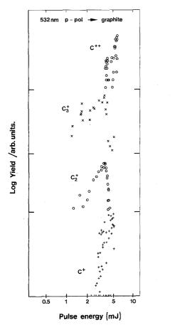
**Fig. 2.** Positive ion yields vs laser pulse energy as measured with the QMS (532 nm, p-polarized light). The  $C_2^+$ ,  $C_3^+$ , and  $C^{++}$  yields have been displaced vertically for clarity
