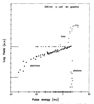
Fig. 1. Electron, photon, and total positive ion yields from a graphite surface vs. laser pulse energy, as measured with the TOF-spectrometer (355 nm, s-polarized light). The electron and ion yields have been displaced vertically for clarity
