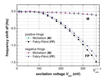
FIG. 3. Frequency shift df plotted as a function of the cantilever excitation voltage  $V_{exc}$  for both fringes of Michelson and Fabry-Pérot interferometer configurations. Strong opto-mechanical interaction is evident in the Fabry-Pérot regime (black squares and blue triangles) but much weaker in the Michelson regime (green and magenta triangles).
