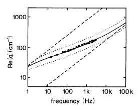
FIG. 3. Measured (circles) and calculated for  $\kappa_f = 1 \text{ cm}^2/\text{s}$  (solid line) thermal wave dispersion curves for a 0.5- $\mu$ m-thick electron beam evaporated gold film on a BK7 glass substrate. Dashed lines show the asymptotic behaviour of the calculated dispersion curve at low and high frequency limits. Dotted curves were calculated for  $\kappa_f = 0.5 \text{ cm}^2/\text{s}$  (upper curve) and 2 cm<sup>2</sup>/s (lower curve).
