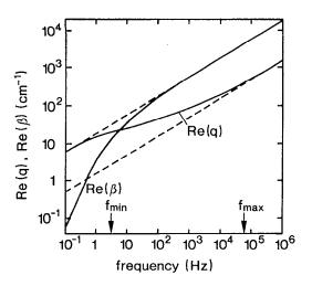
FIG. 1. Thermal wave dispersion curve (real part of the wave number vs frequency) for a 1- $\mu$ m-thick gold film on fused silica. Also shown is the dispersion of Re( $\beta$ ), characterizing the penetration depth of the thermal wave into the substrate. Dashed lines show the dispersion curves for bulk gold (the lower curve) and silica (the upper one) according to Eq. (1).
