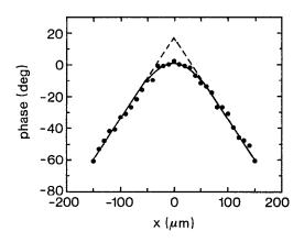
FIG. 2. Phase profile of the surface temperature for a 1- $\mu$ m-thick electron beam evaporated gold film on BK7 glass at 680 Hz. Circles: measured data, solid curve: numerical simulation, dashed lines:  $\Delta \theta = Re(q)\Delta x$ , with qcalculated with Eq. (7).
