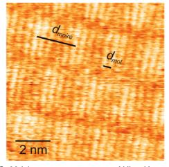
**Figure 5.** Moiré pattern apparent on an arachidic acid monolayer on HOPG exhibiting a periodicity of five molecules (imaging parameters:  $V_b = 0.71$  V and  $I_t = 0.68$  nA). The parameters  $d_{\text{moiré}}$  and  $d_{\text{mol}}$  denote the moiré periodicity distance and the intermolecular distance, respectively.
