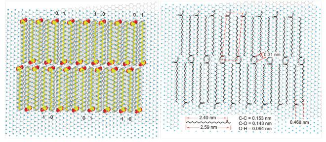
Figure 6. Space-fill and skeleton models for the molecular arrangement of arachidic acid on HOPG (model b in Table 1) superimposed with the hexagonal grid of  $\beta$  carbon atoms of the graphite surface. Bond lengths in the hydrocarbon skeletal chains are drawn to scale. The length of the molecule is determined by a construction based on known bond lengths and bond angles taken from literature.<sup>45,46,51,52</sup>
