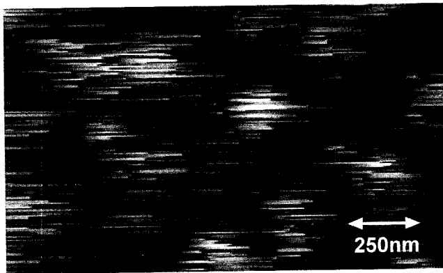
Fig. 2: Contact mode image of colloids. The stripes are a result of the adhesion between tip and metal. The stripe starts when contact is established and ends when the cantilever torsional force exceeds adhesion. The strength of the adhesion can be inferred from the size of the stripes often acting far beyond the extension of the colloid.
