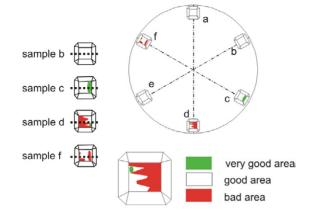
**Figure 1.** Six samples are symmetrically glued on the machining wheel to give all samples the same machining treatment. SFM measurements were performed at various positions along the dotted lines. The classification of 'bad', 'good' and 'very good' areas is a result of visual inspection with a Nomarski microscope.
