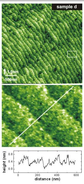
**Figure 4.** Misalignment of the machining plane and the surface of sample d results in the creation of a vicinal surface composed of a large number of aligned, triple-layer height steps. In this example, the surface inclination is about  $5^{\circ}$ . A cross-section was taken in a magnified area enclosed by the white rectangle.
