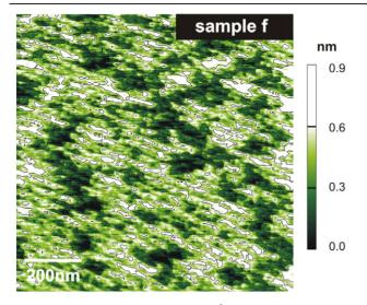
**Figure 3.** Highly resolved image of  $1 \ \mu m^2$  in a good area imaged on sample f that yielded the best machining results. The scale bar covering a range of 0.9 nm reveals that all surface features can be associated with three different height levels separated by steps of 0.3 nm height.
