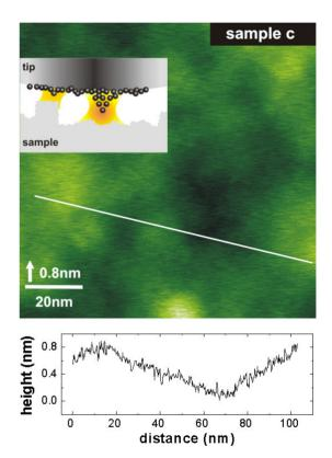
**Figure 6.** Highest resolution image taken in a very flat region of sample c. The size of the apparent surface features is determined by smearing effects due to the finite radius of the tip apex, as schematically illustrated by the inset. An interaction with more than one cluster may contribute to the total tip–sample interaction.
