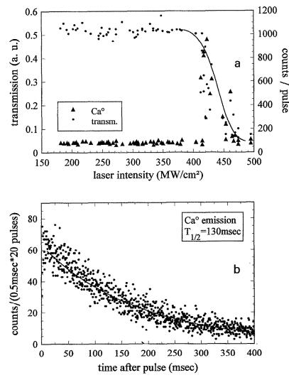
Fig. 3. Type 2 damage spot, irradiated with laser intensities below the ablation threshold. (a) Laser-intensity dependent  $Ca^0$  desorption yield and laser light transmission. (b) Time-of-flight spectrum of the delayed  $Ca^0$  emission signal integrated over 20 pulses in the vicinity of the intensity breakdown threshold.
