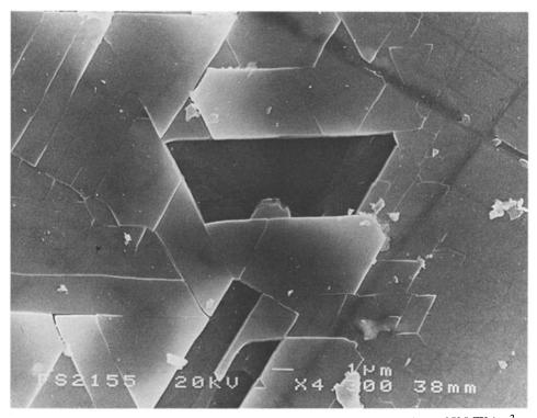
Fig. 4. SEM micrograph of surface damage resulting from single-shot irradiation at 950 MW/cm<sup>2</sup>.
