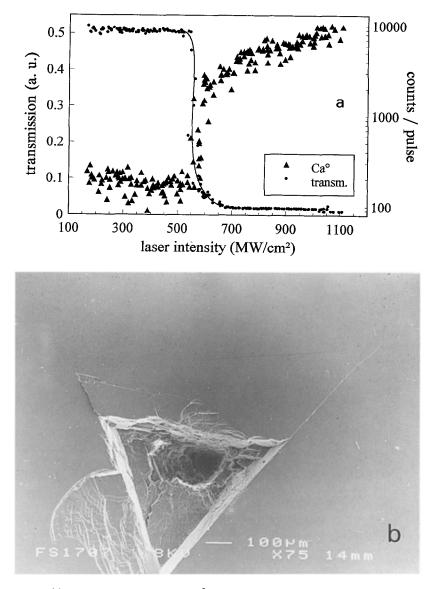
Fig. 1. Type 1 damage spot. (a) Laser-intensity dependent Ca<sup>0</sup> desorption yield and laser light transmission; (b) SEM micrograph of surface damage.
