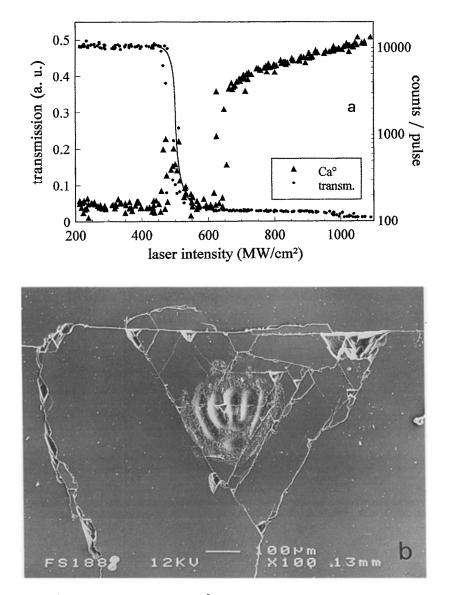
Fig. 2. Type 2 damage spot. (a) Laser-intensity dependent Ca<sup>0</sup> desorption yield and laser light transmission; (b) SEM micrograph of surface damage.
