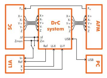
FIG. 1. (Color online) Connections of the drift-compensation (DrC) system with the scan controller (SC), the atomic force microscope (AFM), the lock-in amplifier (LIA), and the computer (PC). The five piezo signals  $X\pm$ ,  $Y\pm$ , Z are high-voltage signals whereas all other connections are low-voltage inputs and outputs.  $F_N$  is the cantilever deflection signal.
