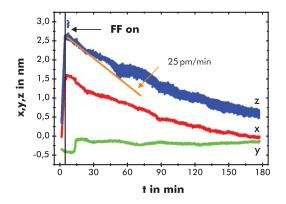
FIG. 7. (Color online) Drift characteristics during the 3D data acquisition on a calcite  $CaCO_3(10\bar{1}4)$  surface. After the feed-forward (FF) is activated with the drift velocities determined by the tracking, the residual drift is 25 pm/min at maximum as indicated by the orange line.
