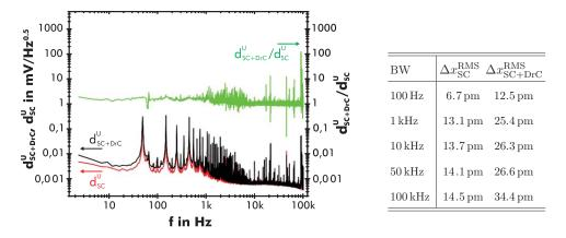
FIG. 3. (Color online) Noise measurement on the high-voltage  $X^+$  output signal of the original scan controller ( $d_{SC}^U$ , left scale) and of the combined scan controller and drift compensation system ( $d_{SC+DrC}^U$ , left scale). The ratio  $d_{SC+DrC}^U/d_{SC}^U$  is referenced to the right scale. In addition, the table lists the piezo dislocation noise for different piezo bandwidths.
