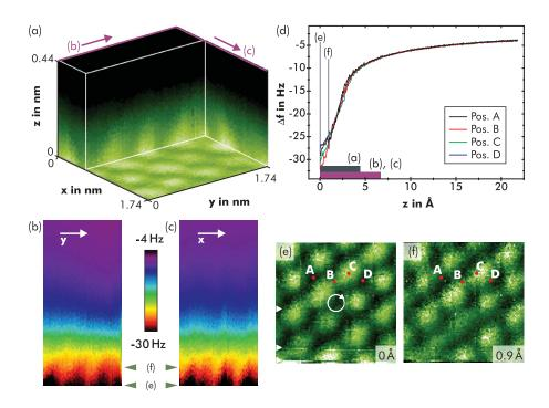
FIG. 8. (Color online) Different representations of the force field above CaCO<sub>3</sub>(1014): (a) presents a cropped 3D view of the data acquired. Planes along different axes are extracted and presented in (b), (c), (e), and (f). Furthermore, it is possible to extract  $\Delta f(z)$  curves from different surface sites as depicted in (d). The trajectory of the circular tip movement is depicted in (e).
