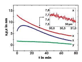
FIG. 5. (Color online) Drift characteristics and positioning precision of our drift-compensation system. Here, a surface species on the  $CaCO_3(10\overline{1}4)$  surface is used as the reference, the drift is measured over about 75 min. Non-linear drift behavior is directly evident and for the *Z* channel, the drift is even non-monotonic.
