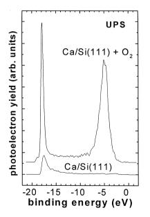
Fig. 4. MIES spectrum of a Ca on Si(111) film (thickness > 20 nm) prepared in the UHV and Ca/Si(111) exposed to ca 300 L oxygen.
