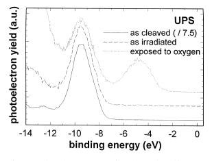
Fig. 2. UV photoelectron spectra of CaF<sub>2</sub>(111) cleaved in UHV, irradiated with 150 mC cm<sup>-2</sup> of 1.5 keV electrons and subsequently dosed with 15 L oxygen at a pressure of  $5 \times 10^{-6}$  Pa. The photoelectron yield for the unirradiated surface was divided by a factor of 7.5 while the other two spectra are shifted upwards in this representation.  $E_{\rm F}$  refers to the Fermi energy of the spectrometer.
