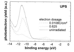
Fig. 1. UV photoelectron spectra of  $CaF_2(111)$  as cleaved in air and after irradiation with different dosages of 2.5 keV electrons at a current density of 180  $\mu$ A cm<sup>-2</sup>. Sample temperature was 400 K during irradiation and 490 K during UPS measurements. For increasing dosage the F 2p intensity decreases while the O 2p peak is formed. The Fermi level is that of the analyser corrected by 1 eV sample charging.
