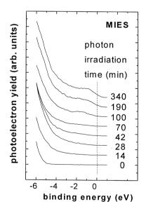
Fig. 3. MIES spectra of the time development of the emission from air cleaved  $CaF_2(111)$  during irradiation by 1486 eV photons. Only the region between the oxygen emission and the Fermi energy is shown.
